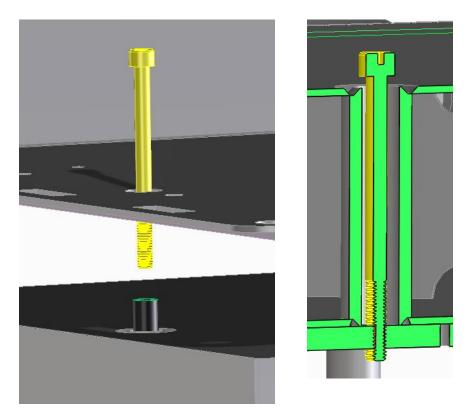
Step 8 Start all bolts with one or two threads.NOTE: Do not tighten any of these 4 bolts until all have been started. Getting everything aligned can be tedious.
