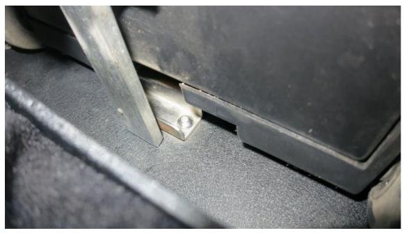
Removal of the case is simply a matter of raising the latch and then giving the case a good tug to disengage the mounting tabs.
