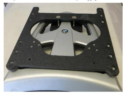
There are stainless steel tabs that engage the forward part of the luggage rack. The rear of the plate has M8 studs which extend through the luggage rack. The plate is locked in place by a clamping plate affixed over the M8 studs.
