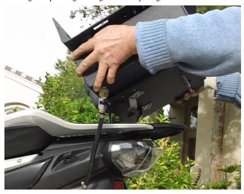
Once in position place the clamping plate over the mounting studs on the rear and install the locking plate as described in LRM Mounting Plate Installation on page 6.
