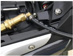
**Note:** It is a good idea to check that you have enough clearance by installing the seat and making sure the hose can slide freely through the slot you have cut.
