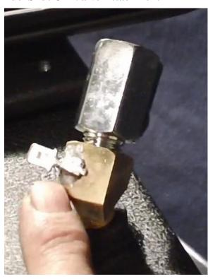
The shut off valve assembly has been assembled but not attached to the tank. Additionally, the tank bung has PTFE paste sealant pre-applied.
